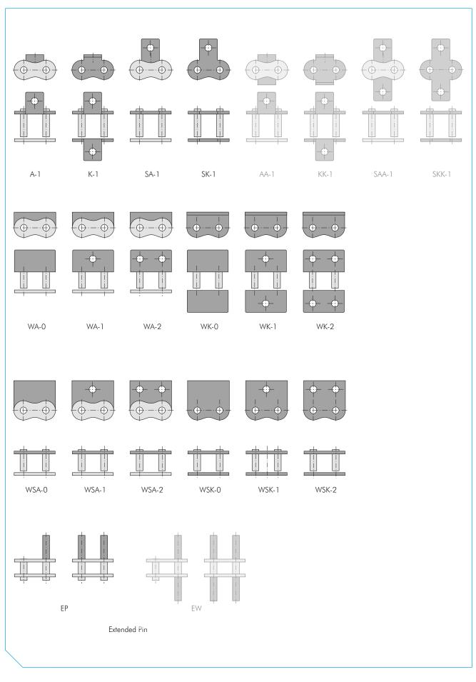
Fig. 3 Overview Single Pitch Attachment Types
