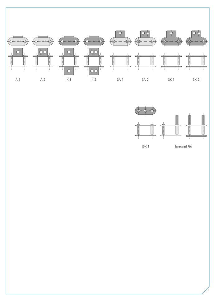
Fig. 4 Overview Double Pitch Attachment Types
